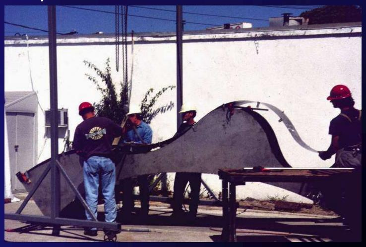
Fitting the cut and formed stainless steel sheets together.
