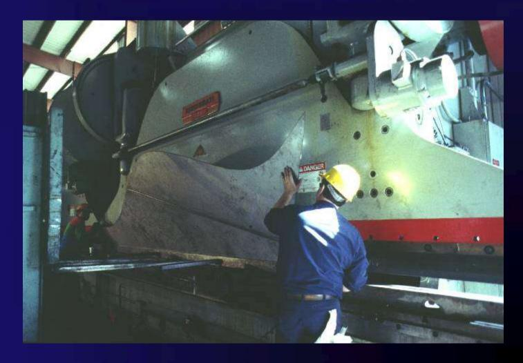
Cut stainless steel is bent with a 300 ton Press Break.
